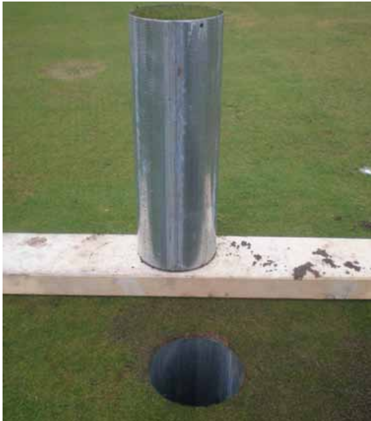
Photo 1a,b. Cylinder installed for measurement of actual ET on green (left) and fairway (right). Photos: Trygve S. Aamlid
