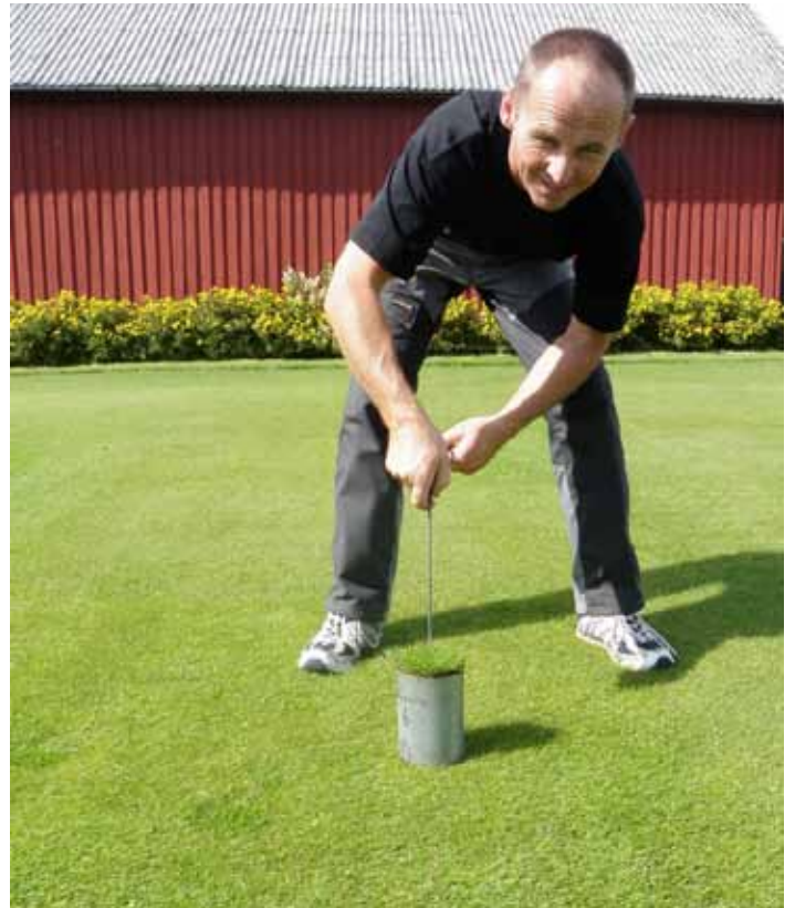
Photo 1a,b. Cylinder installed for measurement of actual ET on green (left) and fairway (right). Photos: Trygve S. Aamlid
