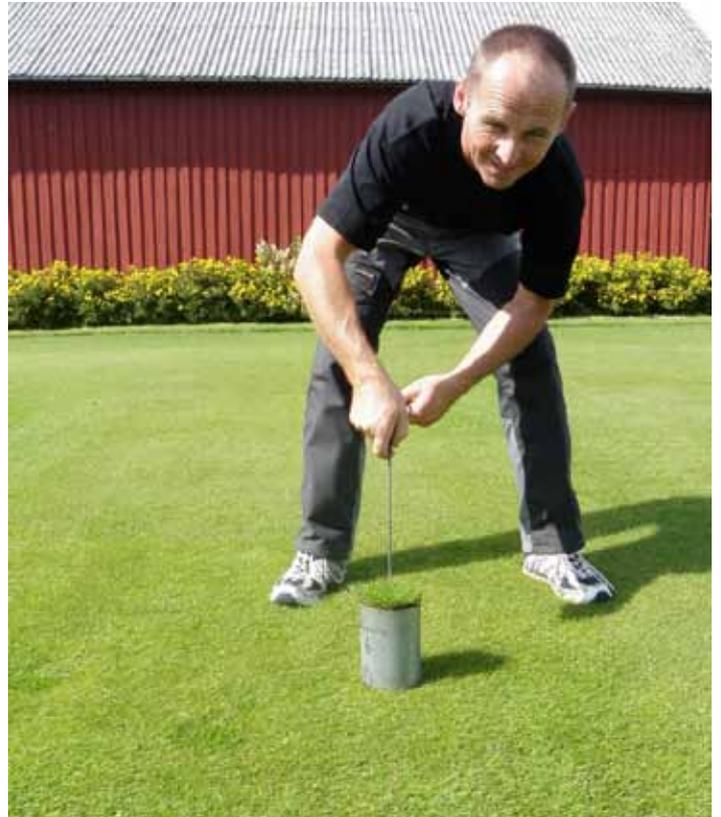
Photo 1a,b. Cylinder installed for measurement of actual ET on green (left) and fairway (right). Photos: Trygve S. Aamlid
