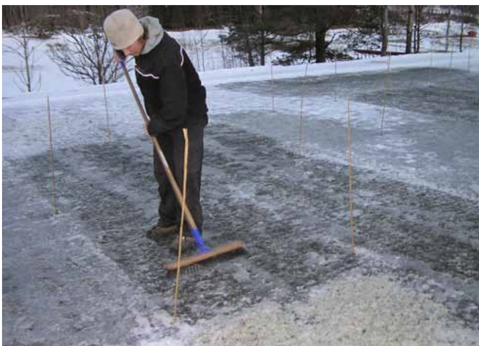
This ice was removed as a part of an experiment. The light green colour of the crushed ice indicates correct working depth. Photo: Agnar Kvalbein, Bærum GC, February 2008
