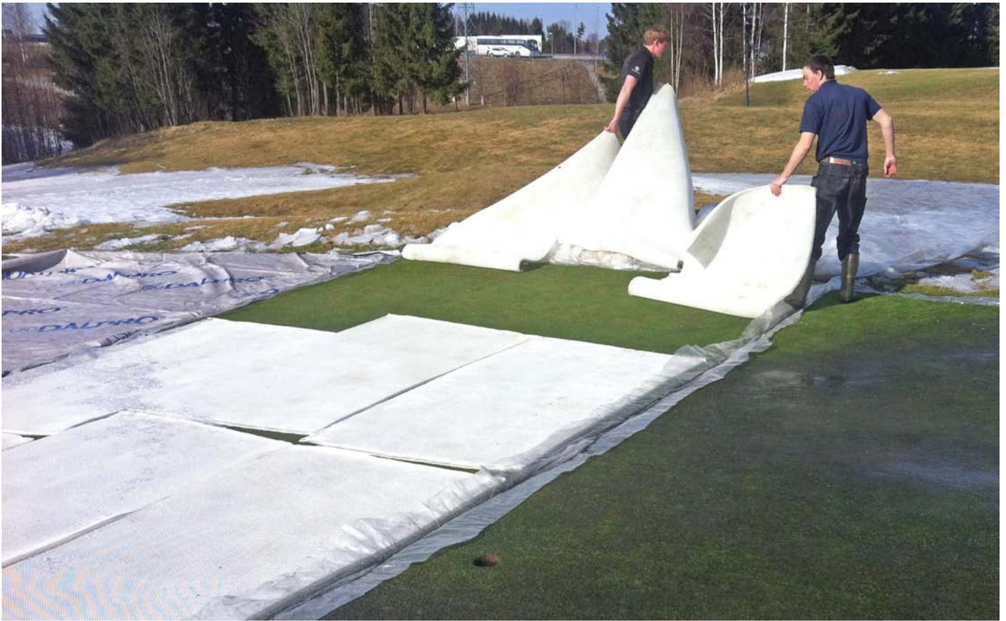
Special fabric creating an 18 mm air filled space between plastic and turf is being removed from a full scale experiment on Miklagard golf course, Norway. To the left is a semi-permeable tarp. The right part was covered with plastic only. Photo: Stefan Schön.
