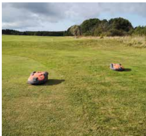
Above: Robotic mowing on fairway and semi-rough at Grenå GC. Photo: Karin J. Hesselsoe.
